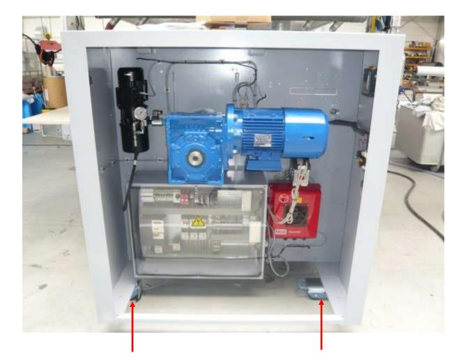
To place the rollers under the machine, the machine can be lifted with a hydraulic jack on these 4 supports.
