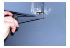
Dismantle the protective plate at the back.
